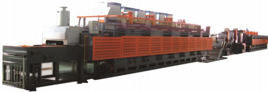
连续式淬火炉 负载运转指示灯 The Continuous Mesh Belt (Carburizing) Furnace Line running sign lamp
