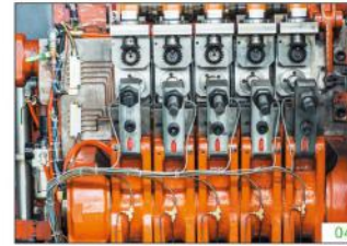
图04为后通机构，各工位后通机构可分为单独调整且最后一个工位可通过调整凸轮位置成更换凸轮实现切边或通出动作，所有机型的通出前死点位置不变，部分机型可选择加装带有数字显示的手轮式或数控后通牙管调整机构。 Fig.04 is rear knock - out mechanism. Rear knock - out mechanism of various stations can be respectively and independently adjusted. Last station can. Before being kicked out, dead - point position of all models keeps the same. Some models can choose to add hand - wheel type or CNC type rear knock - out threaded pipe adjusting mechanism.
