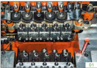
图01为RBF系列多工位零件成形机配置的可反转的螺母类和固定式螺栓类产品夹仔。 Fig.01 reversible nuts and fixed bolt clips that match with RBF serial multi-station parts forming machine.
