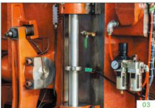
图03为夹仔台往返运动和夹仔的开闭动作均由共同的中间传动轴驱动，可确保动作的协调。 Fig.03 reciprocating movement of clipping table and opening / closing actions of the clips are both driven by a joint intermediate shaft to ensure the coordinated actions.
