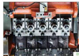
图05为 RBF 系列机型的冲具通出机构，可实现冲具通出与机器清块后识动作同步进行，使工件成形后停留在打模内由后通出机构通出，避免由冲具带出造成变形。前通出位置各工位可单验调整，所有前通出机构均设有通出力过载保护装置。 Fig.05 is punch knock - out mechanism of RBF serial model. Punch knock - out coincides with back action of machine slider. After the work - piece is shaped, it stays in the mould and then being kicked out by rear knock - out mechanism. It avoids being taken away by the punch and then get deformed. Various stations of front knock - out positions can be independently adjusted. All the front lead - out mechanism have knock - out force over - load protection devices.
