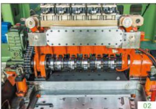
图02为夹料传送为旋摆方式，夹料力为气动并可调，工件传送稳定可靠，适用于机器高速运转。第一工位夹仔遇到送料短寸的可自动张开松料并停机报警。 Fig.02 transfer conveyance of rotary swing mode and transfer force of adjustable pneumatic mode ensures stable and reliable work -- piece conveyance and high speed operation of the machine. The first station clip can automatically loose short dimension feeding, stop and alarm.
