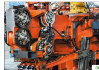
图06为电动式送料机构，棘爪在回程中由气缸自动抬起与棘轮脱离，既可调除摩擦和噪音，又可防止棘轮反转。 Fig.06 is electric feeding mechanism. In return stroke, pawl can be automatically raised by air cylinder and be separated from ratchet wheel. It not only removes friction and noise, but also prevents ratchet wheel from reversal operation.
